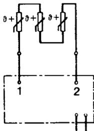
Semiconductor temperature detector with release
